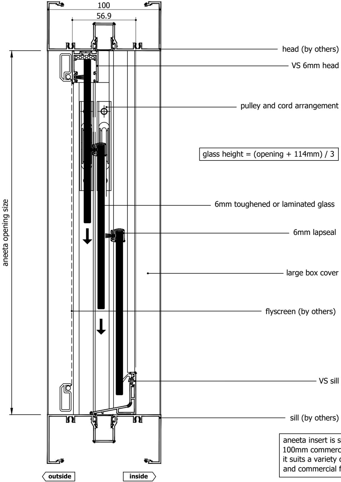
M:\Documentation\Website Downloads\2. Aluminium Frames\1. Vertical\4. Flomotion\MSE 3P6 SSF A (B) - 3 pane 6mm electric Flomotion vertical sliding sery in aluminium frames SSF.dwg
