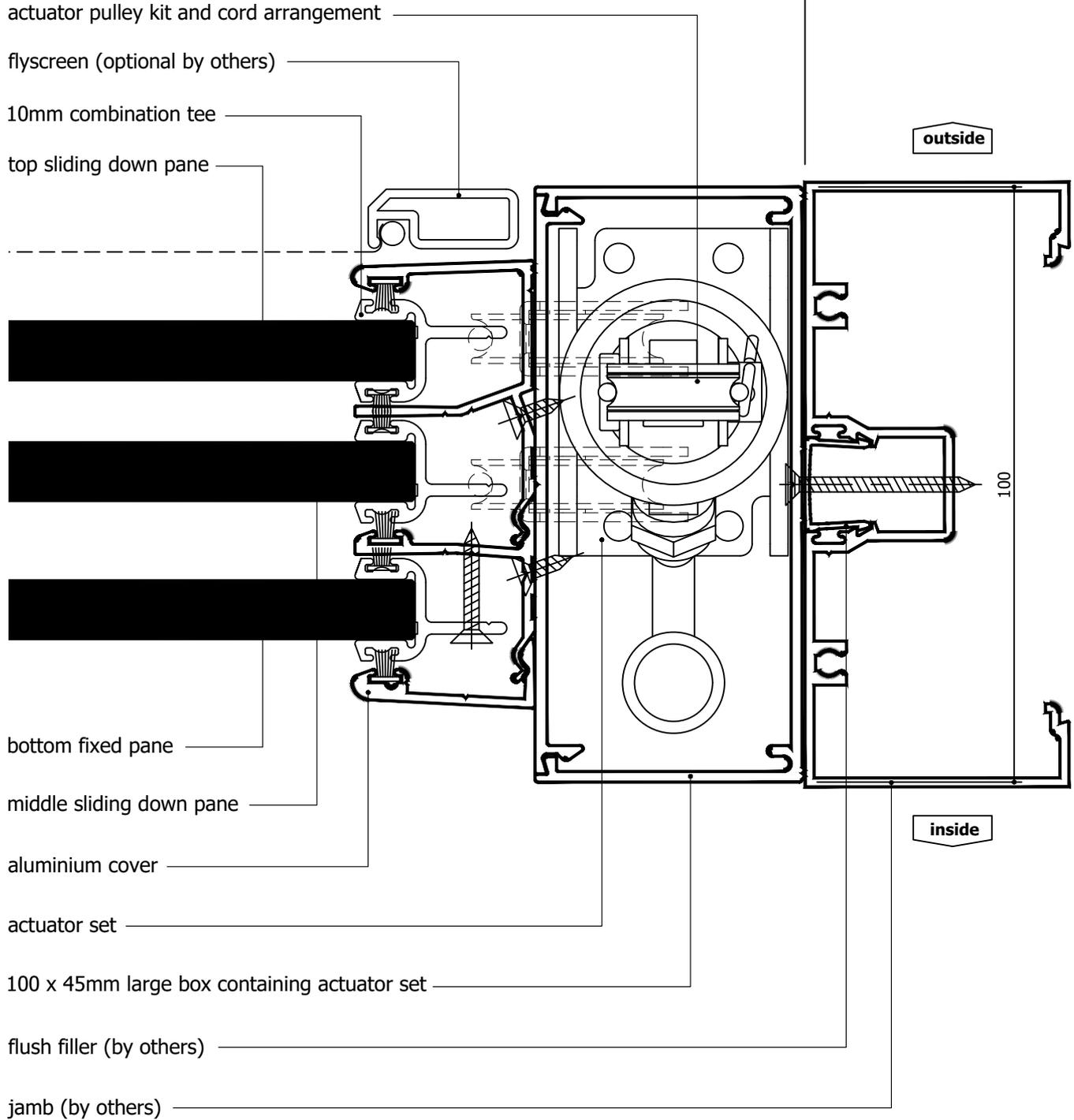
actuator pulley kit and cord arrangement
