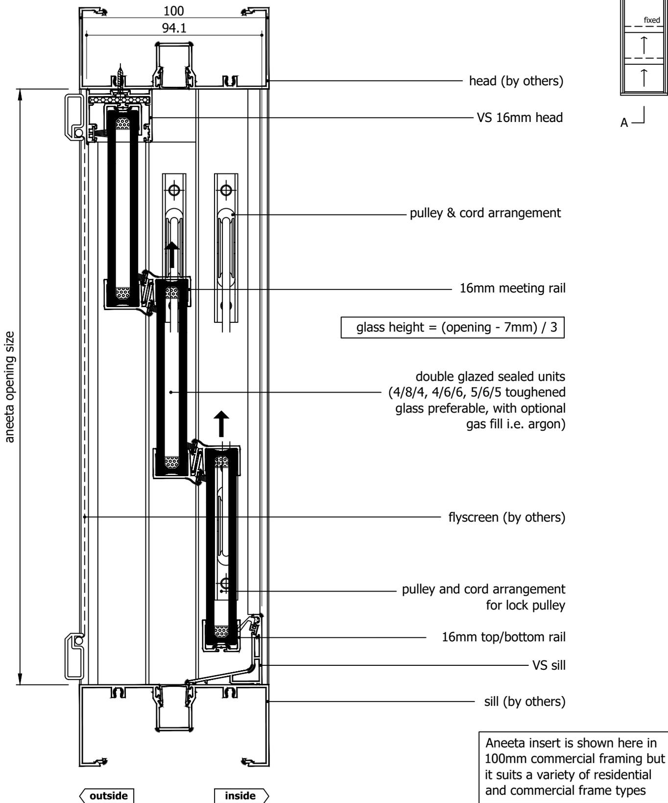
M:\Documentation\Website Downloads\2. Aluminium Frames\1. Vertical\4. Flomotion\MSE 3P16 FSS A (B) - 3 pane 16mm double glazed electric INTERLOCKING Flomotion vertical sliding servery in aluminium frames FSS.dwg
