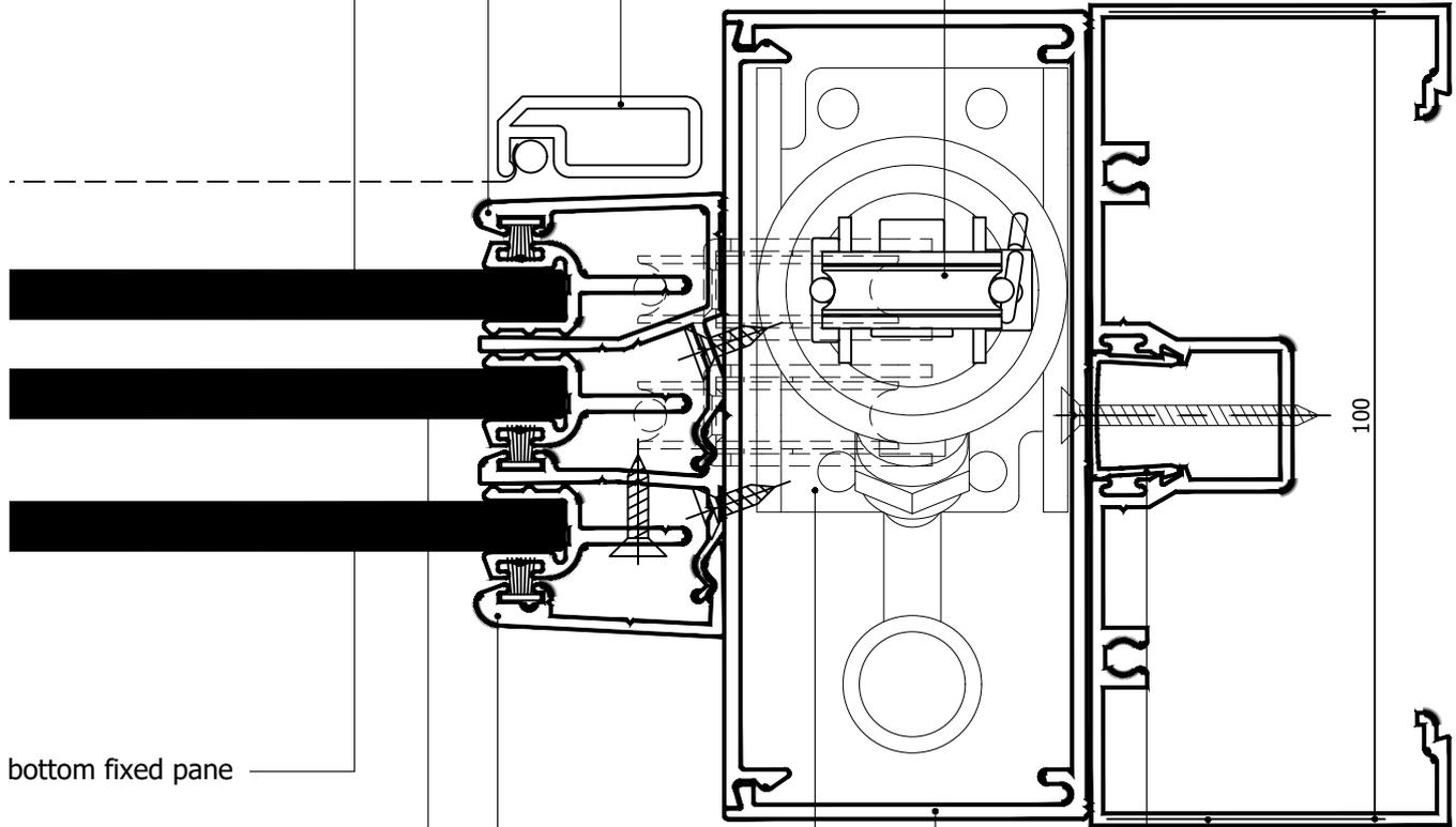
M:\Documentation\Website Downloads\2. Aluminium Frames\1. Vertical\4. Flomotion\MSE 3P6 SSF A (B) - 3 pane 6mm electric Flomotion vertical sliding sery in aluminium frames SSF.dwg
