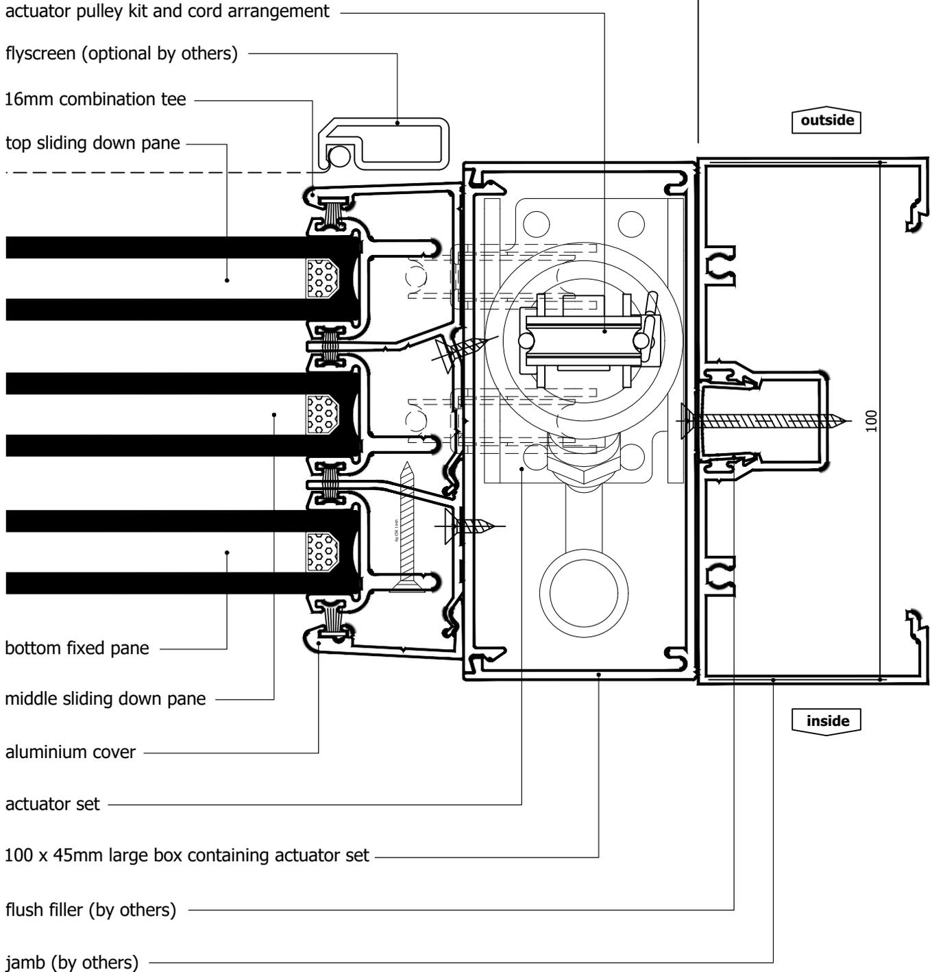
actuator pulley kit and cord arrangement
